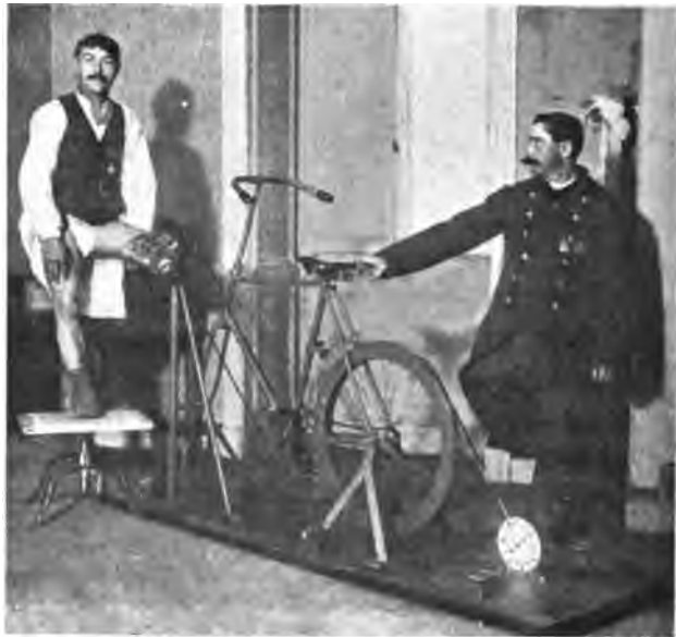
FIG. 80.—Measuring the power of a Stump (Leg) by means of the Dynamometrical splint.
